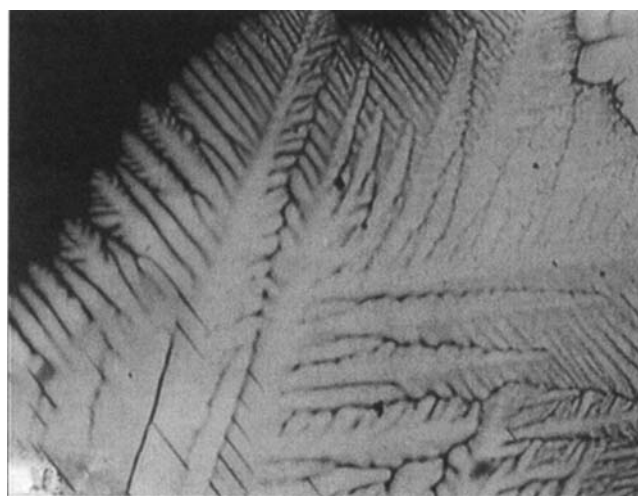
Figure 2. Growth of the M_x phase from the isotropic liquid ( 235^\circ\text{C} , magnification: 100\times ).
