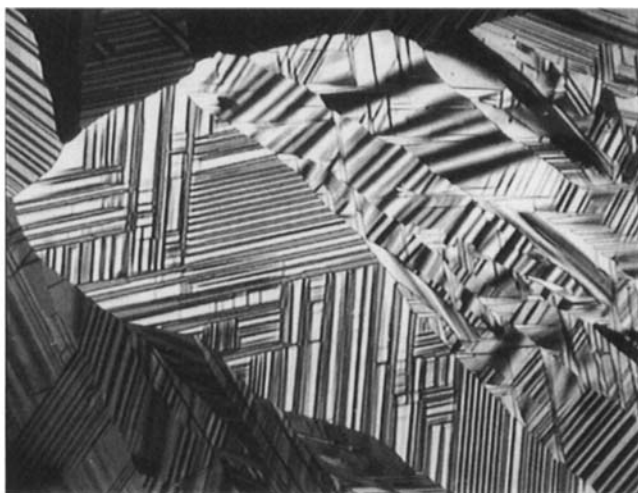
Figure 6. Multi-domain texture of the M_x phase at 190^\circ\text{C} (magnification: 100\times ).
